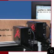
Ability to run up to two printheads from a single controller.
